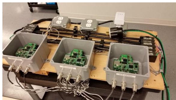
Fig. 3. Belkin Echo hardware being tested in an experimental 3-phase configuration.
